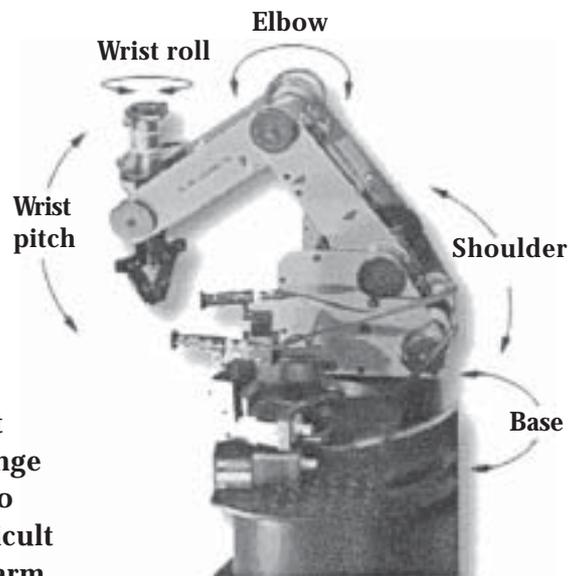
This type of flexibility makes the robot's value much greater and its capabilities attractive. The grippers are at the end of the wrist. They are used to hold whatever the robot is to manipulate. Some robots have end-of-arm tools instead of grippers. A few examples of these tools are painters, arc welders and spot welders. All these put together make a manipulator. This enables a robot to pick up an object, manipulate it, and set it down where desired.
