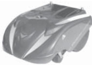
This robot will mow the lawn. Mowbot is equipped with bump sensors which are activated when it encounters an object; it then moves in the opposite direction.
